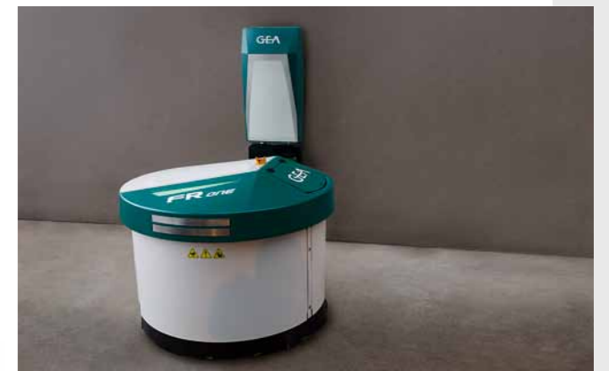
The GEA FRone returns to its charging station automatically and can leave the station either forwards or backwards.
